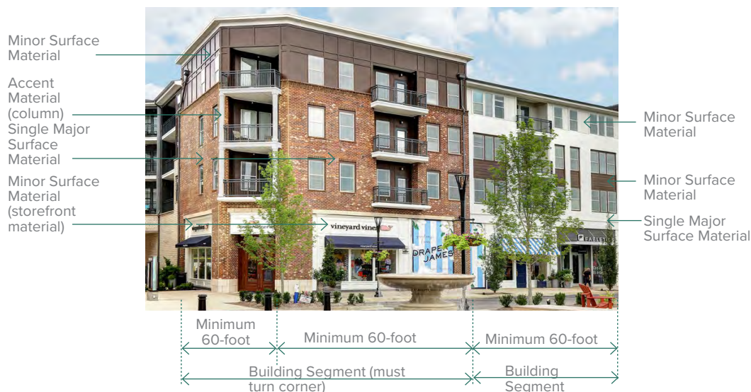
Figure 5-A. Major and Minor Materials on a Facade
